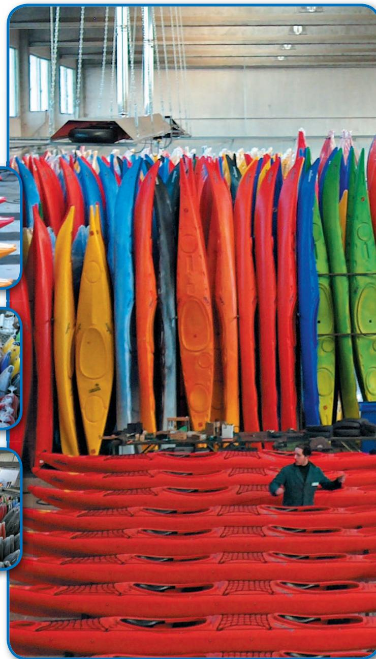
● \*All kayaks are made from our proprietary plastic HDTP. With HDTP we are able to offer you the stiffness or a blow-molded kayak, and the impact resistance of crosslink without either limiting our ability to mold complex shapes, or using materials which are hazardous to the workers.
